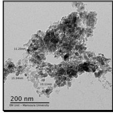
Nano silicon Nano graphite Fig (1) Fig (2) Fig 1,2: TEM imaging of the prepared nanoparticles.
