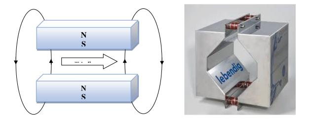
Fig. 1: Schematic of magnetic fields and direction of water flow during the magnetic treatment.
